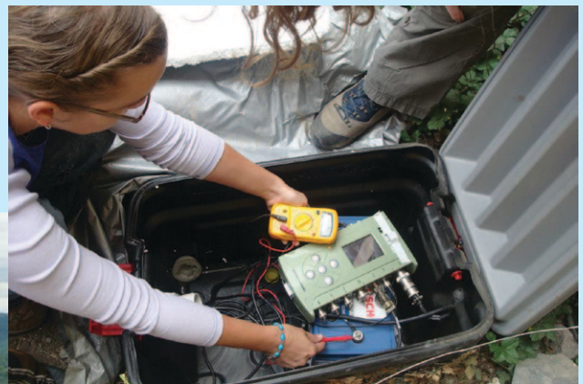
Reading the record stored at a seismic station.
